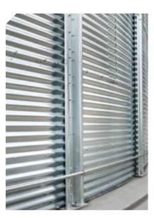
**G115 galvanizing** of stiffeners provides up to 27% longer life. Stiffeners are ASTM A653 Grade 55 with 55K yield and 70K tensile (except 18 gauge).
