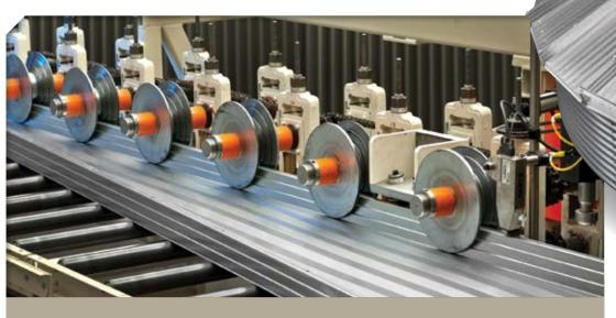
**Proprietary state-of-the-art roll former** controls the distance between holes from rib-to-rib, not from the edge of the coil like competitive products. The result: Higher quality roof sheets that fit better—with bolt holes that line up every time. Bolts drop right in place. That means trouble-free, labor-saving, frustration-free installation on site
