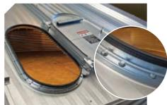
Large pre-formed manway roof opening is standard, featuring a hinged lid and big 5.5 sq. ft. (0.51 m²) opening for easy access. Easy-open lid with big beefy hinges lays flat to avoid wind. Seamless extruded collar (inset) with rubber gasket provides moisture-tight seal when closed. Pre-formed opening makes for simpler construction and tight fit.
