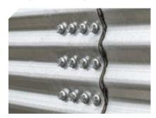
**Grade 8.2 bin bolts** are used throughout to ensure strength and stability. Roofs use 5/16" (0.79 cm) bolts and sidewalls use 3/8" (0.95 cm) bolts.
