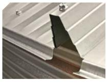
Extra-tall 3-3/4" (9.5 cm) stair-stepped ribs are staggered to provide even greater strength. Hemmed drip edge deflects moisture, eliminates sharp edges to reduce injury and strengthens the cross-section of the roof sheet.
